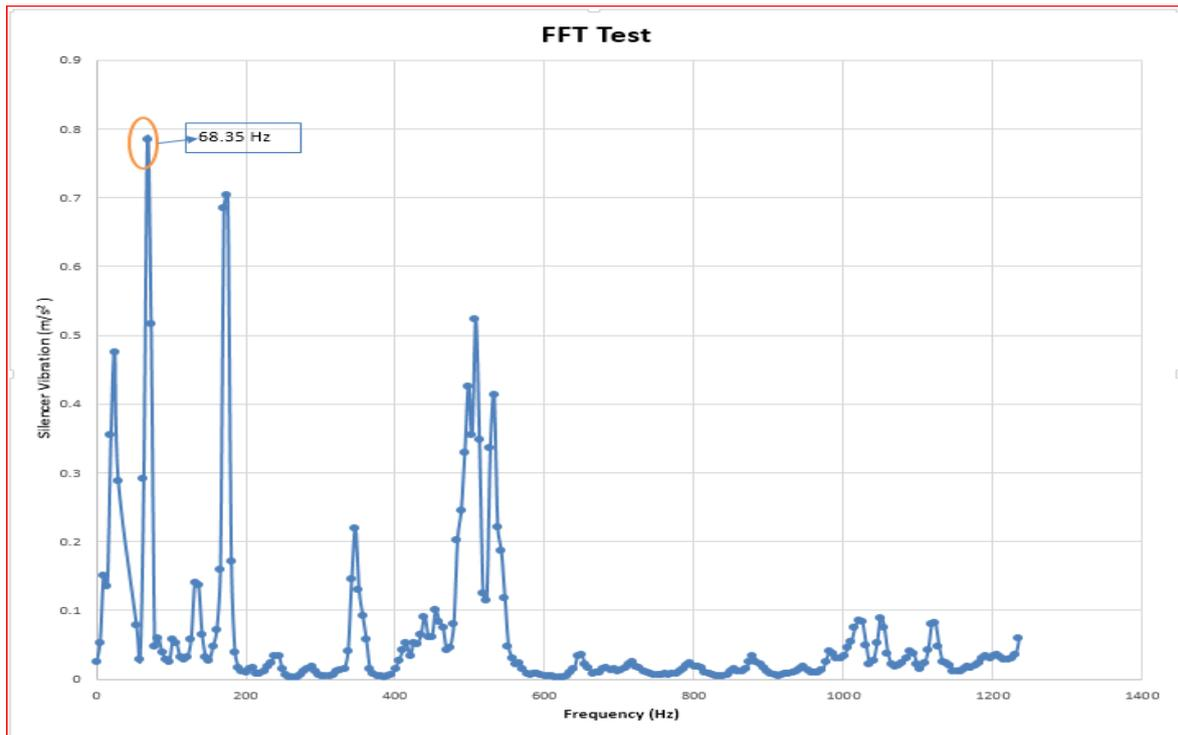
Figure 6. Frequency response showing different mode
