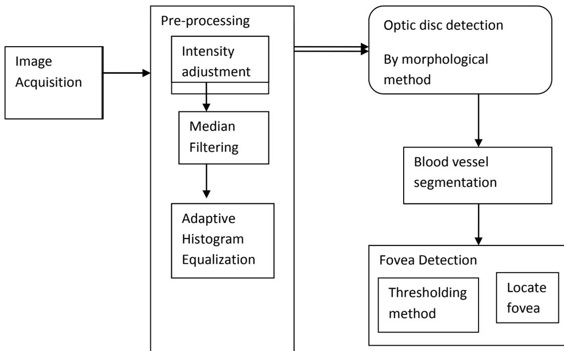
Figure 2 Block diagram for adaptive thresholding method
