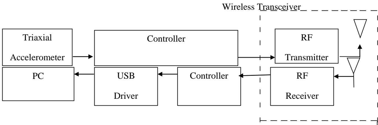
*Fig.1 Block diagram of the digital pen module*
