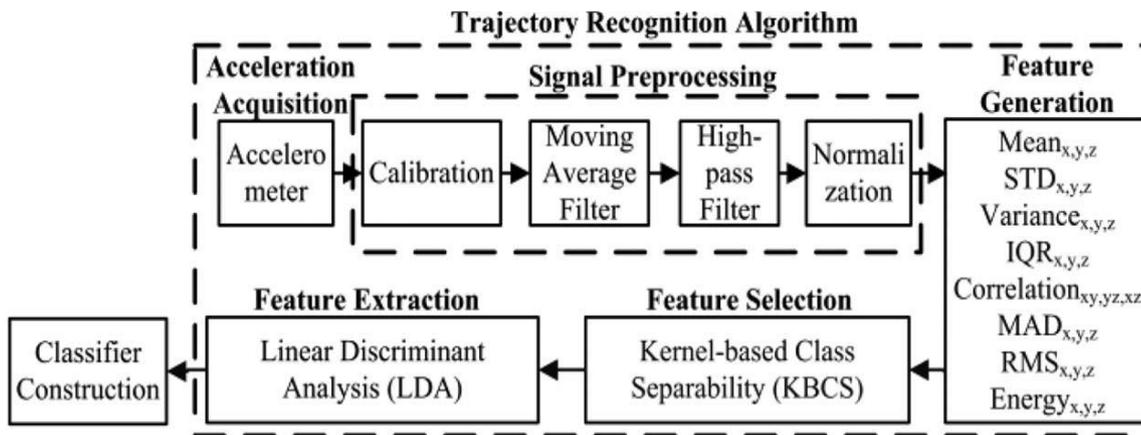
Fig.2 Block diagram of the trajectory recognition algorithm.
