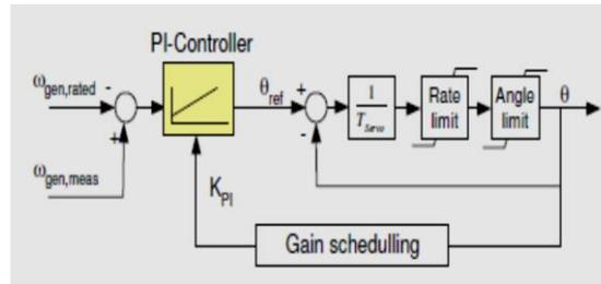
Fig.4. Pitch Angle Control Model
