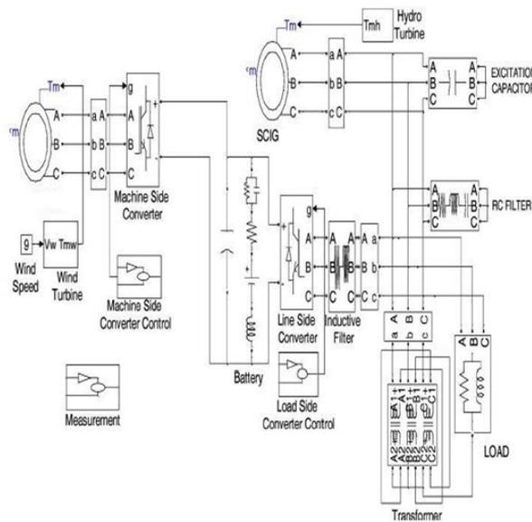
Fig.1. Schematic diagram of wind hydro hybrid system
