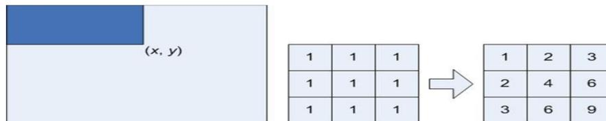
Figure: Integral image generation. representation.
