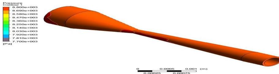
Figure 3.2 pressure of the convergent-divergent nozzle
