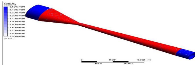
Figure 4.4 velocity of the convergent-divergent nozzle
