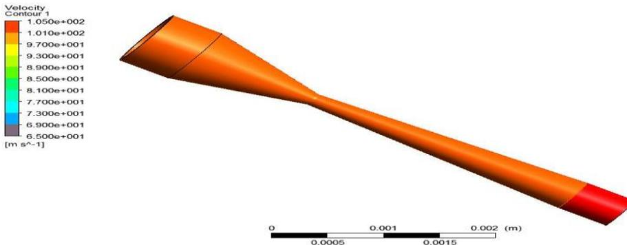
Figure 3.3 velocity of the convergent-divergent nozzle
