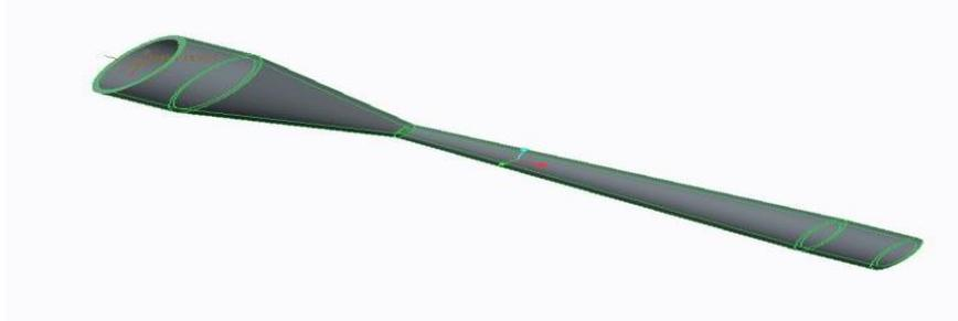
Figure 3.1 Modelling for convergent-divergent Nozzle.
