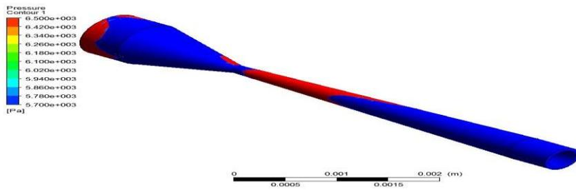
Figure 4.3 pressure of the convergent-divergent nozzle
