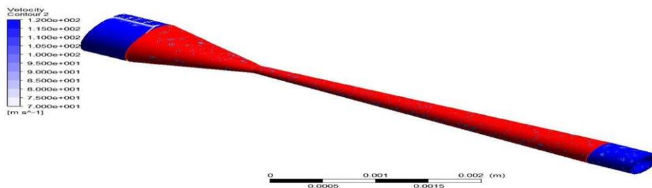
Figure 4.5 velocity of the convergent-divergent nozzle
