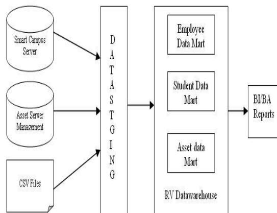
Fig. 1. Engg\_Data warehouse architecture
