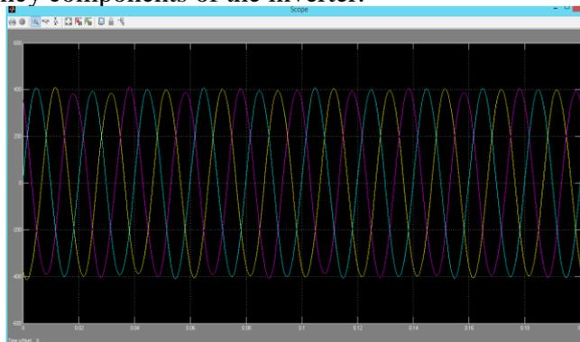
**Fig. 7. Simulation results for Terminal voltages after compensation using proposed hybrid topology.**
