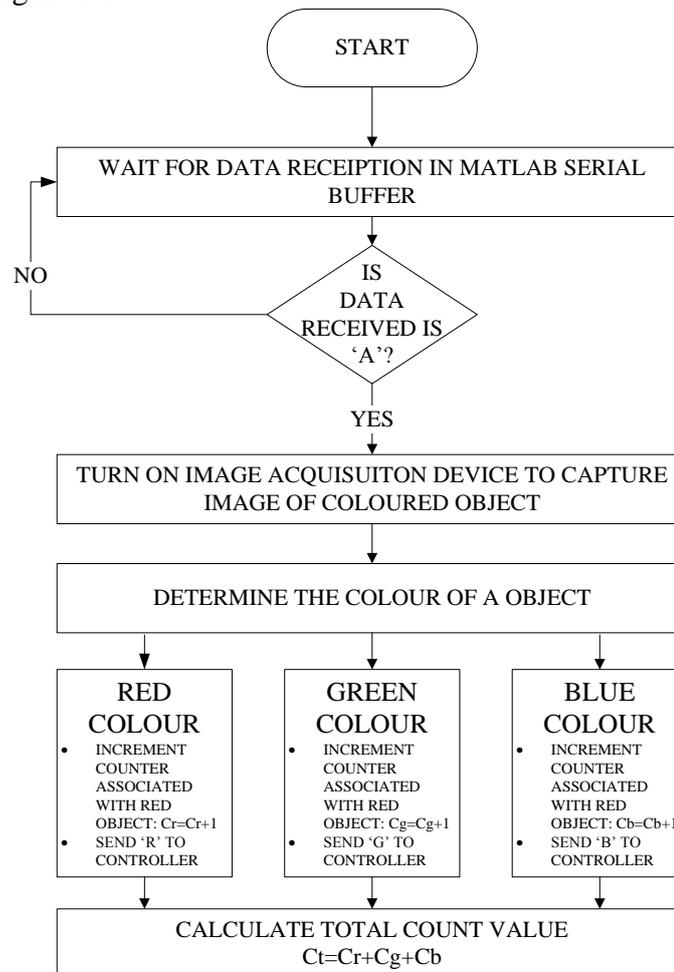
Figure3.5 work flow for object colour and count determination
