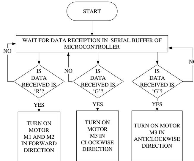
Figure 3.6 flow diagram for object sorting Mechanism
