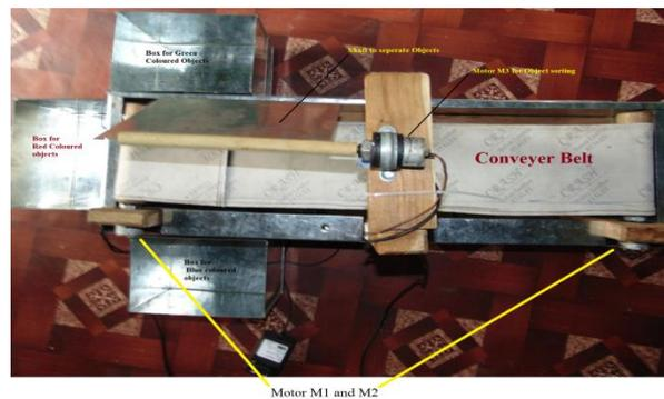
Figure 3.3 Complete hardware view of implemented system
