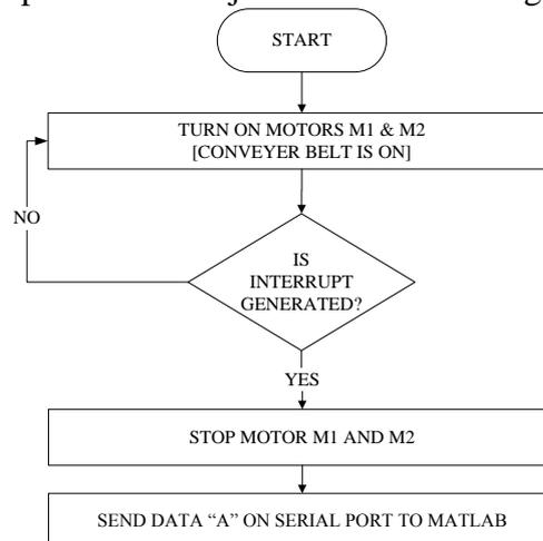
Figure 3.4 flow diagram to sense presence of object
