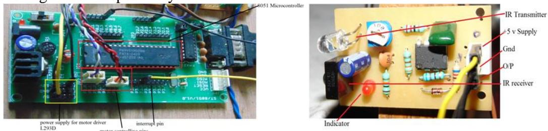
Figure 3.2 (a) 8051 based Controlling unit
