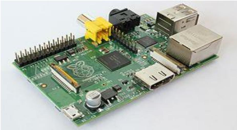
Fig.2.Raspberry Pi ARM11 Single chip Computer
