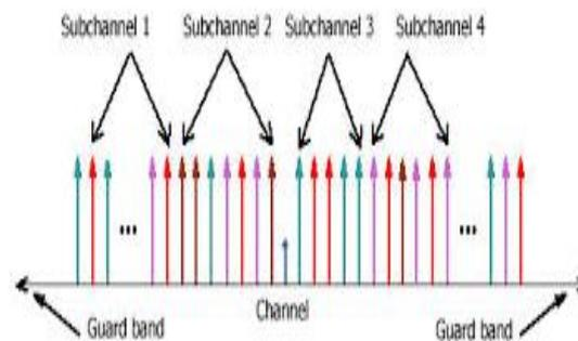
Fig. 3. Example of OFDMA subchannels.
