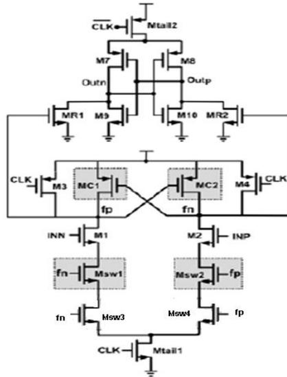
Figure.4. Modified dynamic comparator
