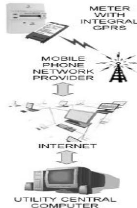
*Fig 1: GPRS Enabled AMR*
