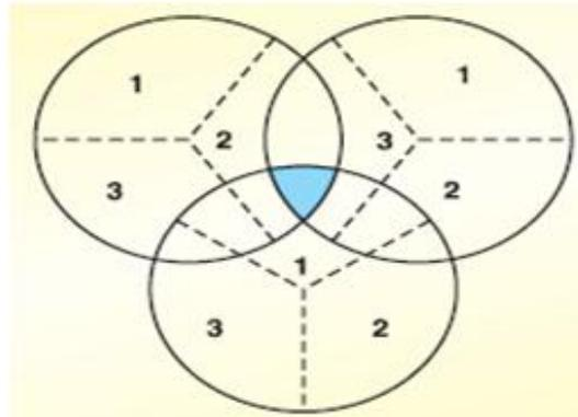
**Fig. 2: The concept of three-way soft hand off**
