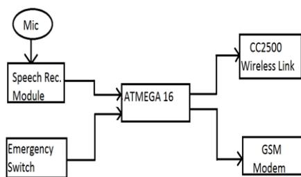
Figure 2. Block diagram of Transmitter
