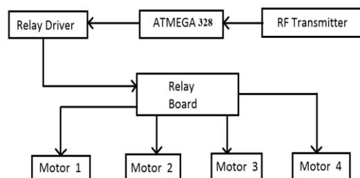
Figure 3. Block diagram of Receiver
