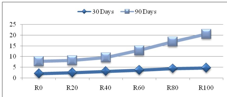
Figure 5.0 % Loss in compressive strength
