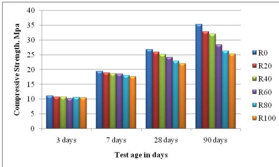
Figure 2: Compressive strength of mixes
