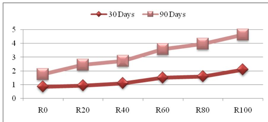
Figure 4.0 % Loss in mass in acid
