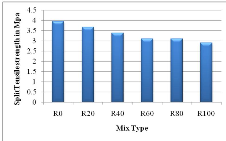
Figure 3: Tensile strength of mixes
