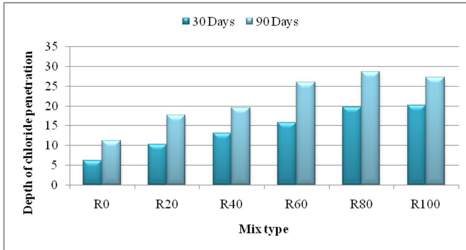
Figure 6.0 Results of chloride ingress
