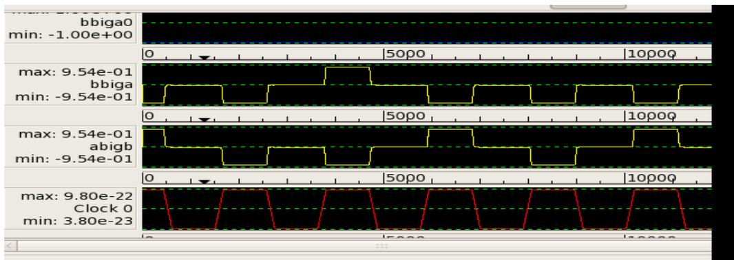
A QCA clock consists of four phases which are called Switch, Hold, Release, and Relax. During the Switch phase, the inter-dot barriers are slowly raised and the QCA cells become polarized according to the state of their drivers (that is, their input cells). During the Hold phase, the inter-dot
