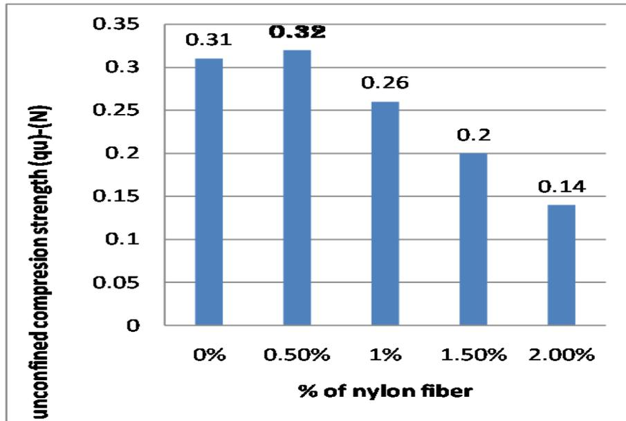
Fig. 2 The UCS values of the soil mixed with fly ash & nylon fiber
