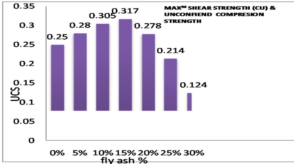
Fig. 1 The UCS values of the soil mixed with fly ash
