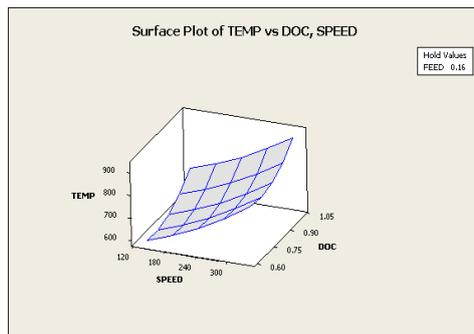
Figure 17(a). Surface Plot of Temp Vs doc, Speed for SAE-8620
