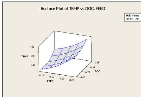
Figure 14(a). Surface Plot of Temp Vs doc, Feed for EN-8
