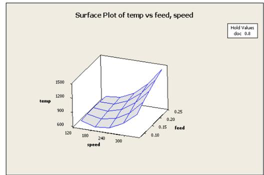
Figure 8(a). Surface Plot of Temp Vs Feed, Speed for SS-316
