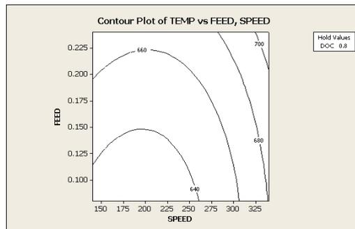
Figure 12(b). Contour Plot of Temp Vs Feed, Speed for EN-8
