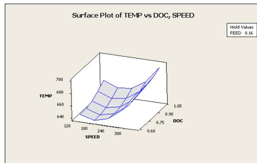
Figure 13(a). Surface Plot of Temp Vs doc, Speed for EN-8
