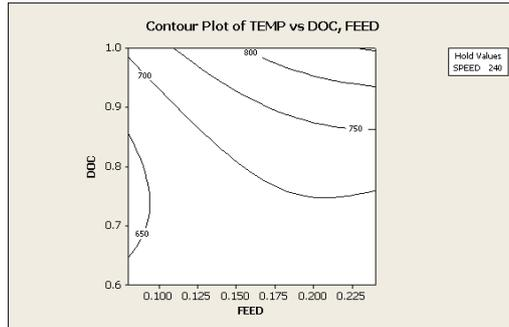
Figure 18(b). Contour Plot of Temp Vs doc, Feed for SAE-8620
