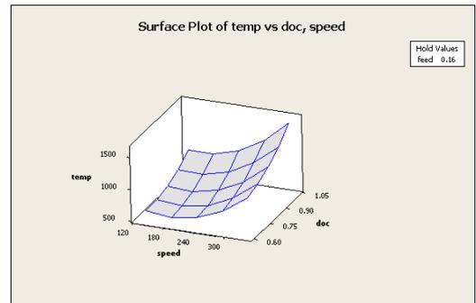
Figure 9(a). Surface Plot of Temp Vs doc, Speed for SS-316
