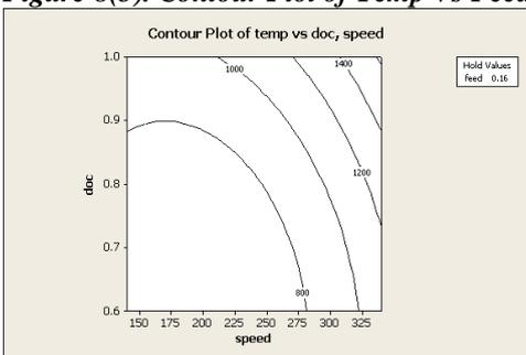
Fig. 9(b). Contour Plot of Temp Vs doc, Speed for SS-316
