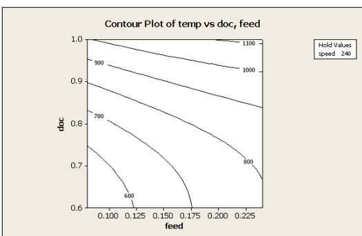
Figure 10(b). Contour Plot of Temp Vs doc, Feed for SS-316
