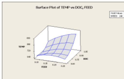
Figure 18(a). Surface Plot of Temp Vs doc, Feed for SAE-8620
