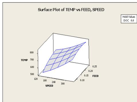
Figure 16(a). Surface Plot of Temp Vs Feed, Speed for SAE-8620
