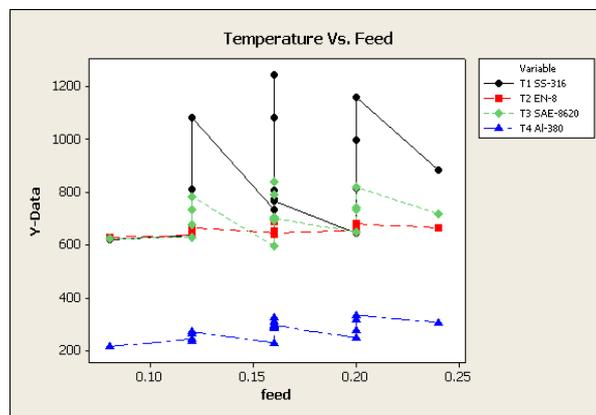
Figure 24. Temperature Vs Feed of materials according to their thermal conductivity
