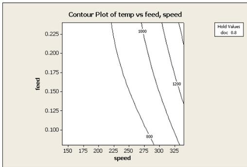
Figure 8(b). Contour Plot of Temp Vs Feed, Speed
