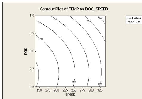
Figure 17(b). Contour Plot of Temp Vs doc, Speed for SAE-8620
