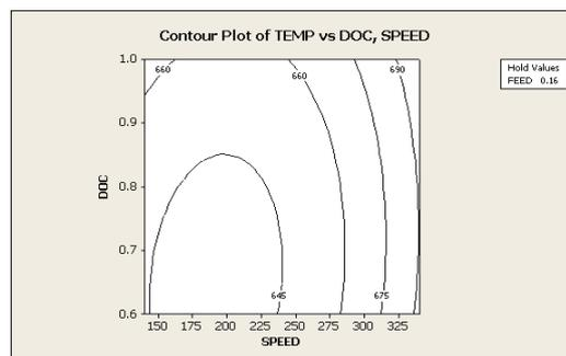
Figure 13(b). Contour Plot of Temp Vs doc, Speed for EN-8
