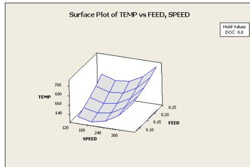
Figure 12(a) Surface Plot of Temp Vs Feed, Speed for EN-8
