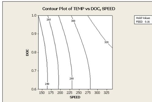
Figure 21(b). Contour Plot of Temp Vs doc, Speed for Al-380
