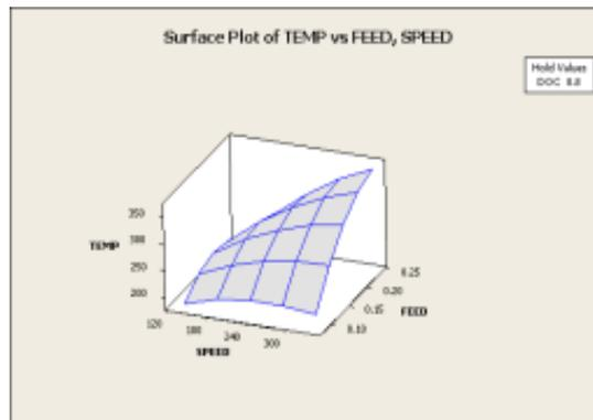
Figure 20(a). Surface Plot of Temp Vs Feed, Speed for Al-380
