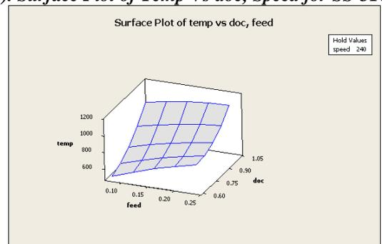
Figure 10(a). Surface Plot of Temp Vs doc, Feed for SS-316
