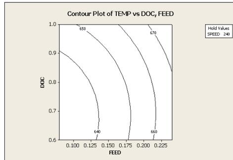
Figure 14(b). Contour Plot of Temp Vs doc, Feed for EN-8
