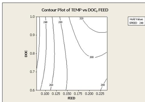
Figure 22(b). Contour Plot of Temp Vs doc, Feed Al-380
