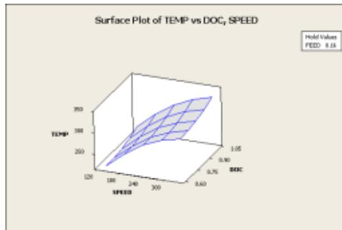
Figure 21(a). Surface Plot of Temp Vs doc, Speed for Al-380
