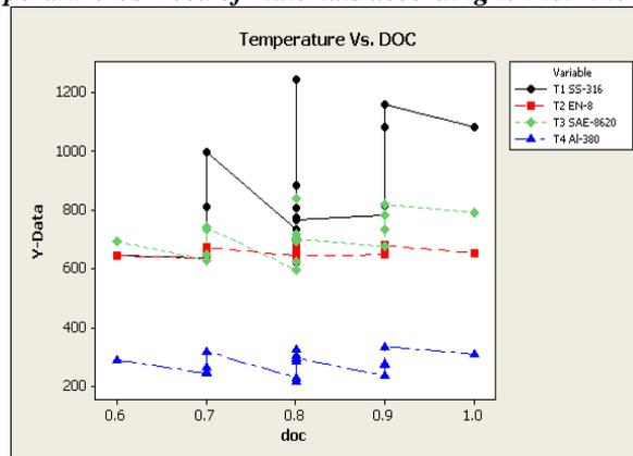
Figure 25. Temperature Vs Depth of cut of materials according to their thermal conductivity
