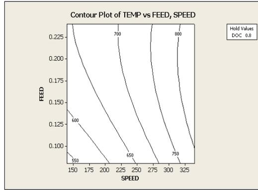
Figure 16(b). Contour Plot of Temp Vs Feed, Speed for SAE-8620
