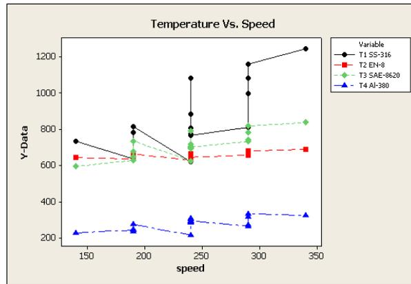
Figure 23. Temperature Vs Speed of materials according to their thermal conductivity
