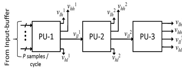
Figure 7. Proposed structure for computation of three level 2 D DWT
