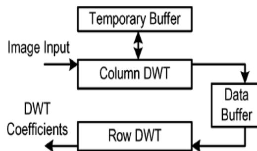
Figure 4. General line-based scheme for single-level column-row 2-D DWT
