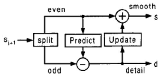
Figure 2. Lifting based implementation
