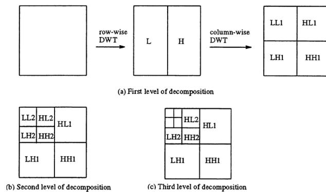
Figure 6. Three level decomposition of 2 D DWT
