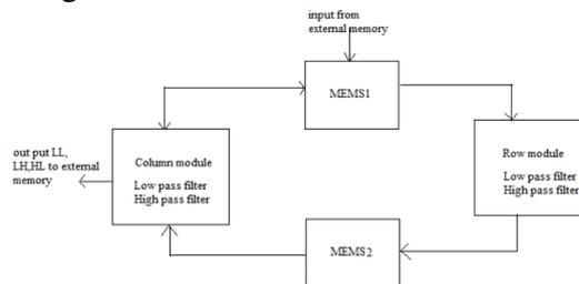
Figure 3. Convolution based architecture
