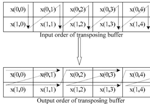
Figure 5: Input and output scanning method of transposing buffer based on parallel scanning method
