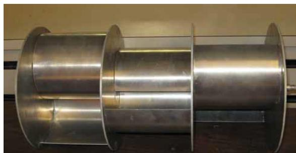
Fig 5: Three Stage Savonius Rotor [11].
