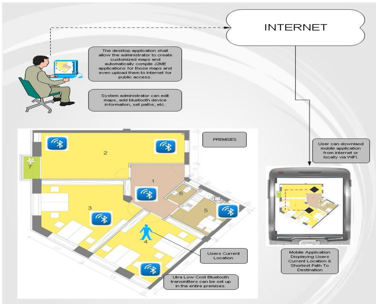
*Fig 3: Architectural Block Diagram of Indoor Navigation System*
