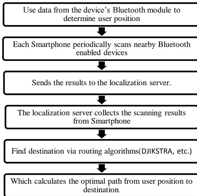
*Fig4:-Flow of indoor positioning system.*
