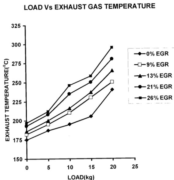
Figure 3. Effect of EGR on Exhaust Gas Temperature
