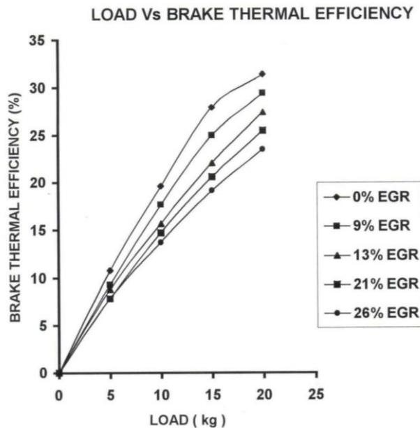
Fig 4. Effect of EGR on Brake Thermal Efficiency
