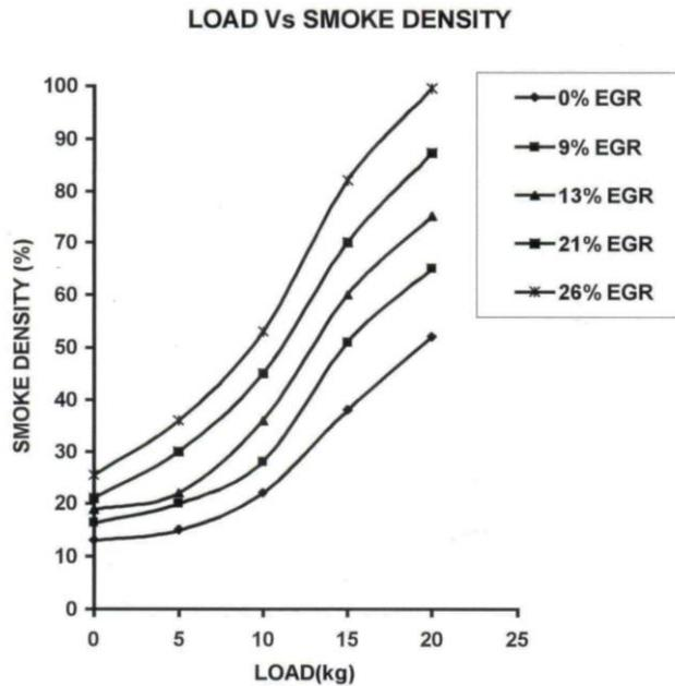
Fig 5. Effect of EGR on Smoke Density
