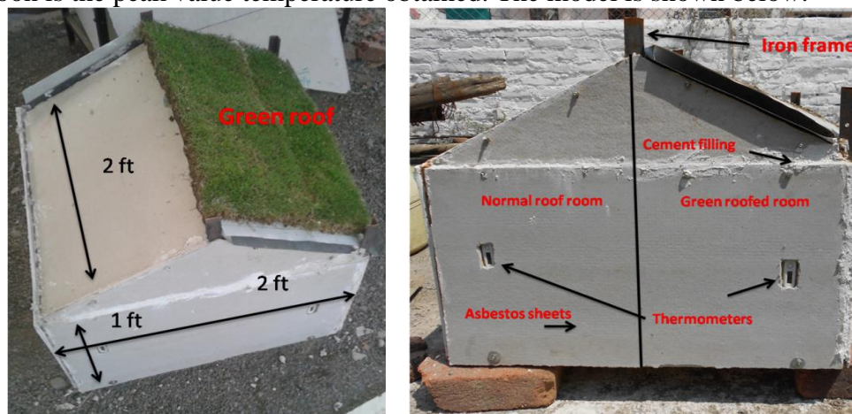
Fig. 2 - Green roof model
