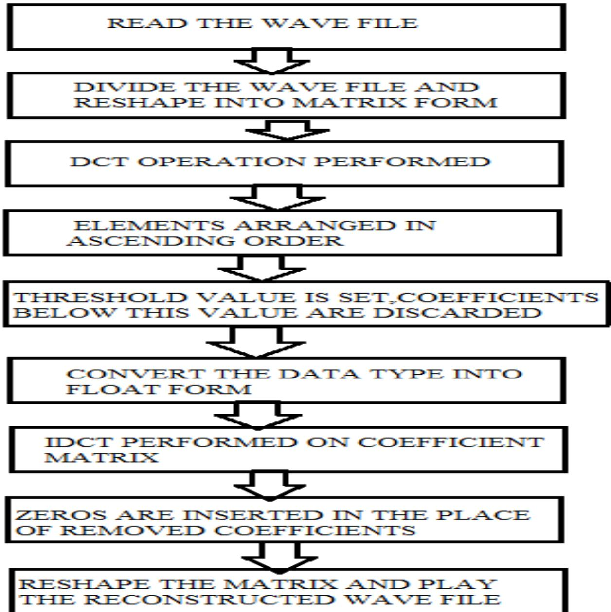
Fig.2: DCT based speech coder design flow
