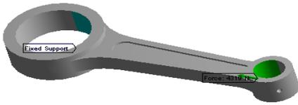
Fig. 2.3 FEA model of the connecting rod with axial compressive load at the piston pin end and crank end restrained.
