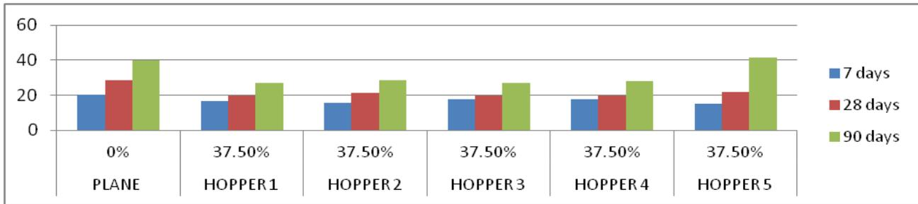
**Graph 3: compressive strength of 37.5% replacement of fly ash mortar**
