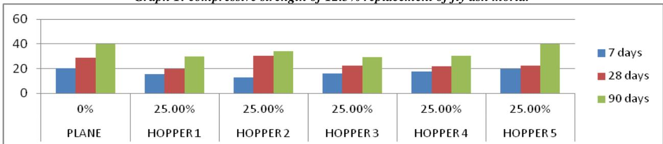
Graph 2: compressive strength of 25% replacement of fly ash mortar
