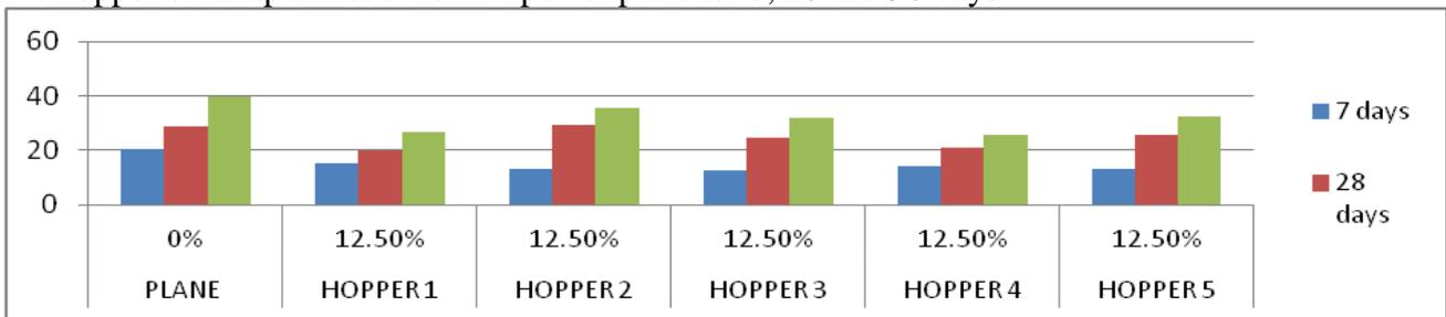
Graph 1: compressive strength of 12.5% replacement of fly ash mortar
