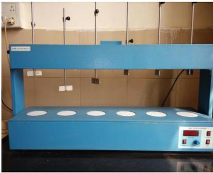
Figure 1. Jar-Test Apparatus
