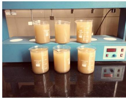
Figure 2. Jar-Test Apparatus with samples
