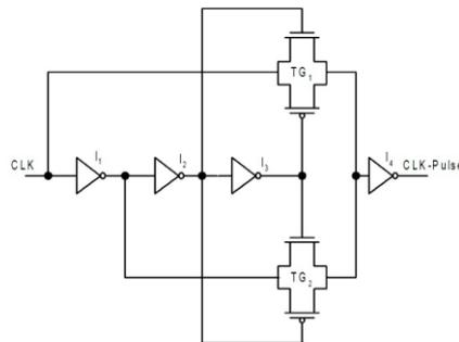
Fig.1 Circuit for Dual-pulse generation
