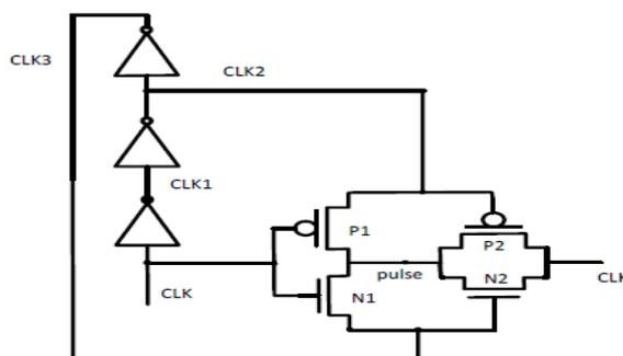
Fig.8 Dual-edge triggered pulse generator
