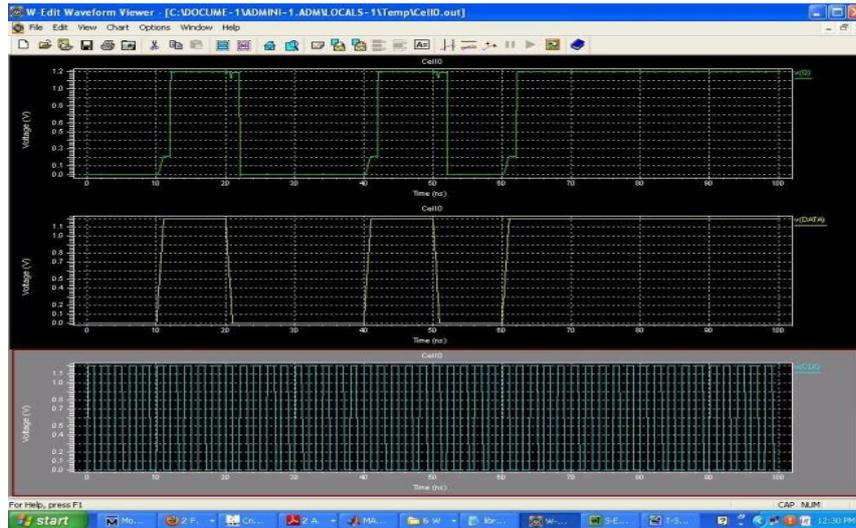
Fig.3 Output waveform of ep-DCO
