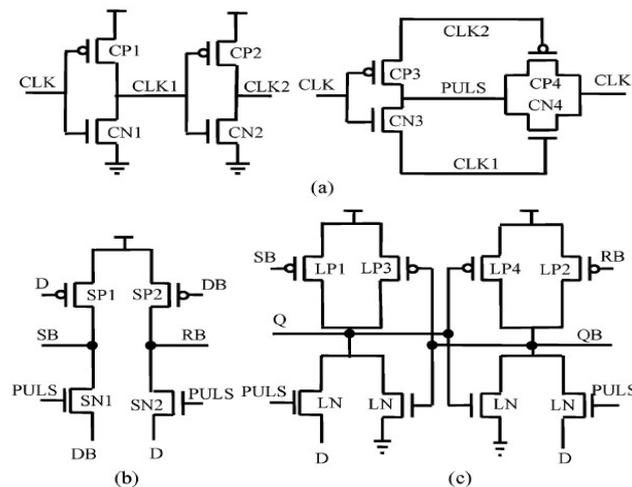
Fig.4 Dual edge-triggered sense-amplifier FF:(a) dual pulse generator (b) sensing stage (c) symmetric latch.
