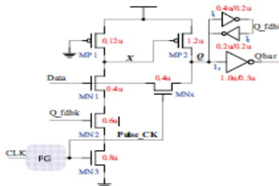
Fig.10 Circuit of proposed P-FF
