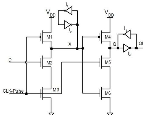
Fig.2 Explicit-pulse data-close-to-output FF
