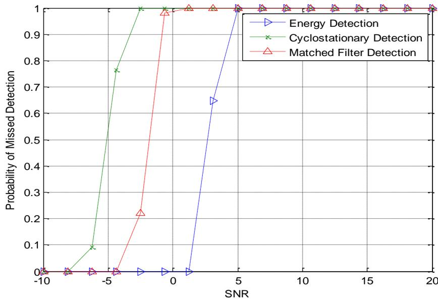
Figure 3. Probability of missed detection Vs. SNR for Matched filters detection, Energy detection and Cyclostationary feature detection.
