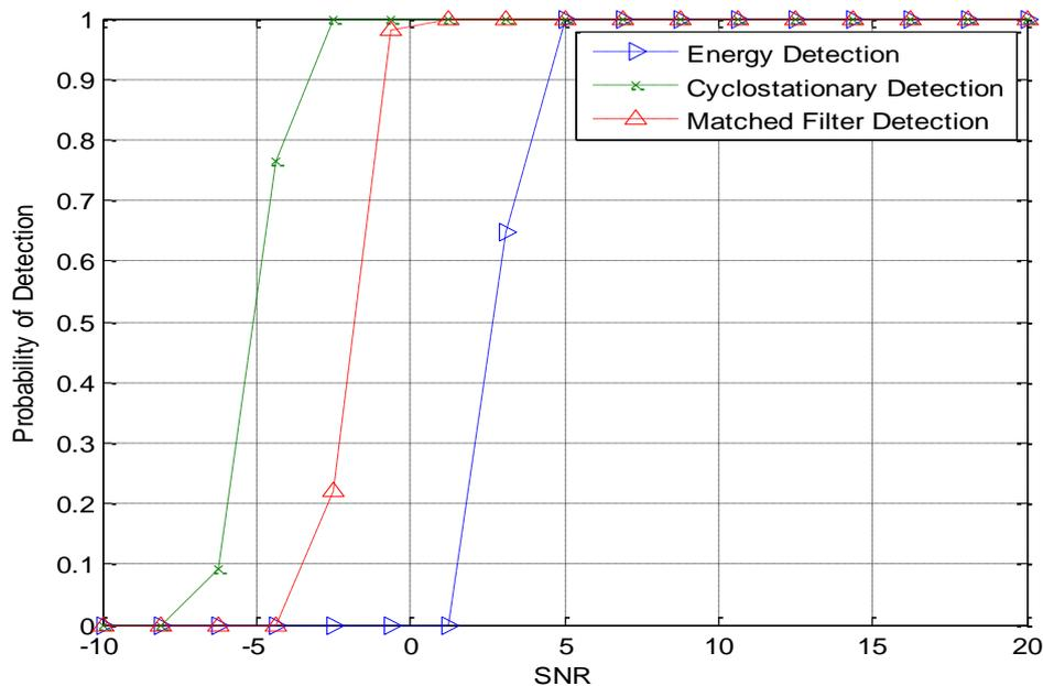
Figure 2. Probability of detection Vs. SNR for Matched filters detection, Energy detection and Cyclostationary feature detection.
