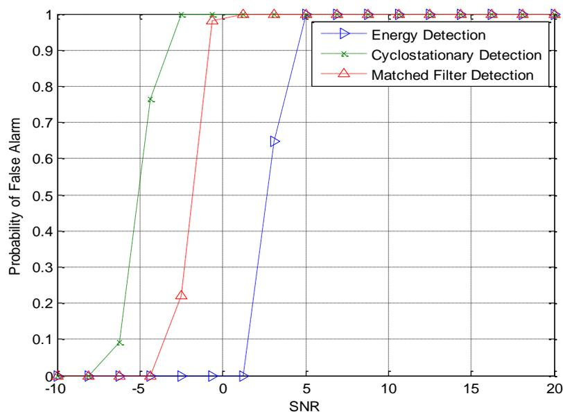
**Figure 4. Probability of false alarm Vs. SNR for Matched filters detection, Energy detection and Cyclostationary feature detection.**
