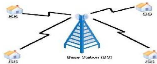
Fig shows the WiMAX network architecture.
