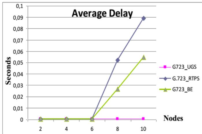
Fig 5(b): Average Delay for G.723 Codec under various service classes
