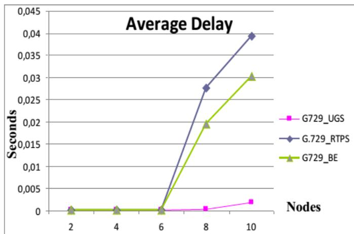
Fig 5(c): Average Delay for G.729 Codec under various service classes
