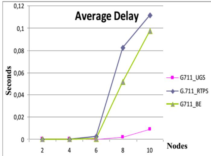
Fig 5(a): Average Delay for G.711 Codec under various service classes
