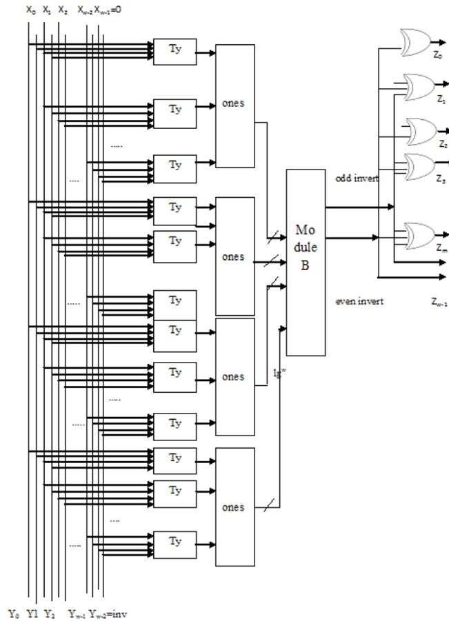
Figure 5 Modified encoder architecture
