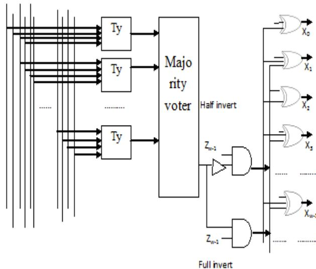
Figure 4 Internal view of decoder block
