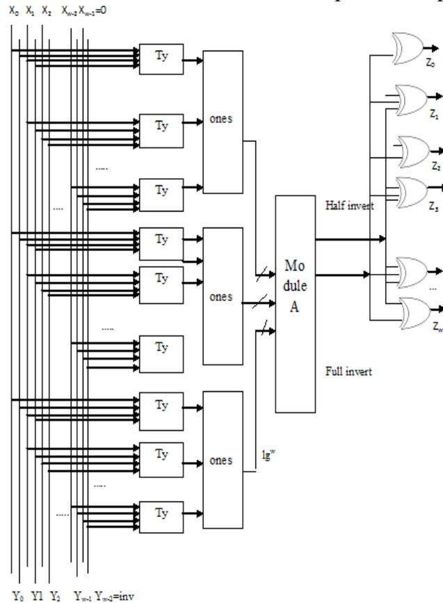
Figure 2 Internal view of encoder block
