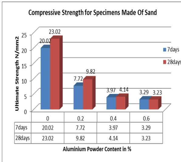
**Fig 1: Compressive strength for sand**
