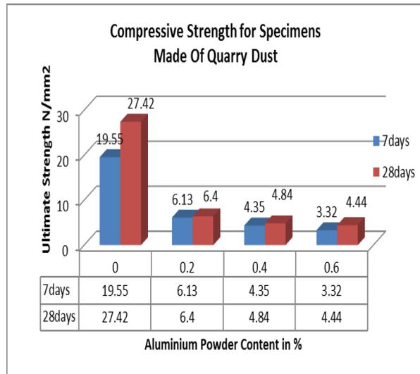
**Fig 2: Compressive strength for Quarry dust**
