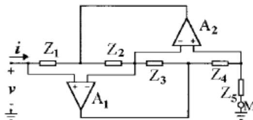
*Figure 2. Antoniou's general impedance converter schematic (Leuciue and Goras, 1998).*
