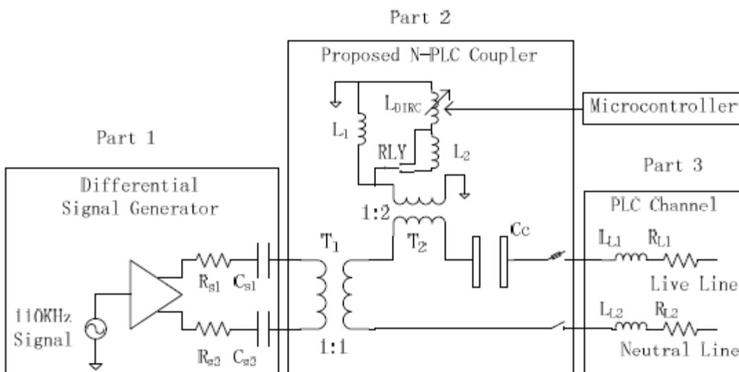
*Figure 1. Adaptive impedance matching network designed in Sun and Amaratunga (2011).*
