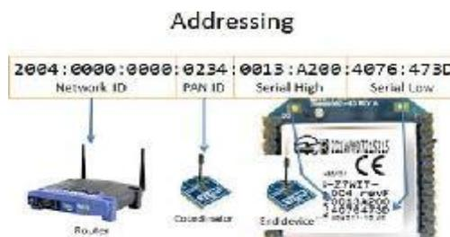
*Fig. 8. Address transformation from ZigBee sensing unit to Internet packet.*
