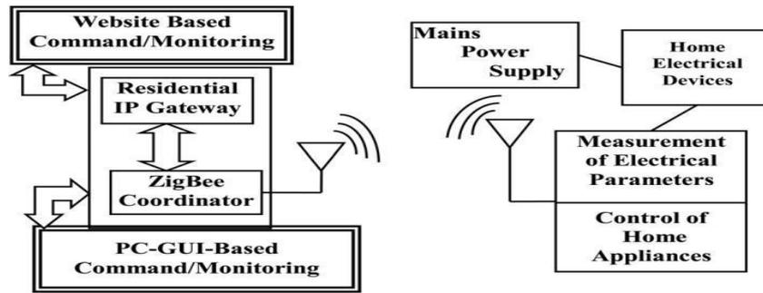
*Fig.1. Functional block diagram of the system.*
