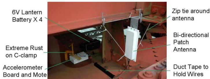
**Fig 4: Placement of actual system for SHM in GGB**
