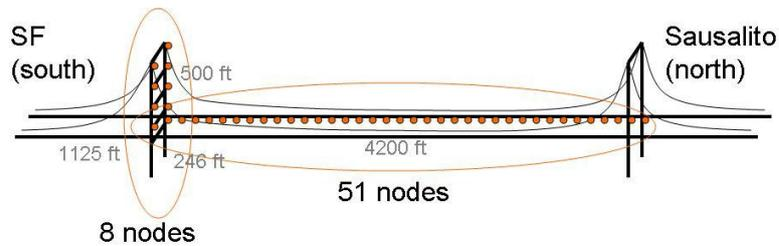
**Fig 3: The Golden Gate Bridge and layout of nodes on the bridge**
