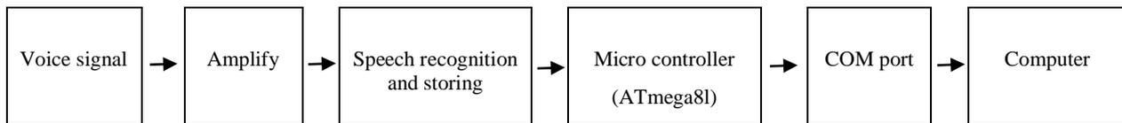
*Figure 2. Circuit Diagram*
