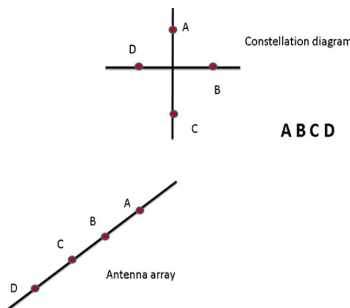
*Figure 1. Mapping of symbols into constellation points and unique antenna positions*
