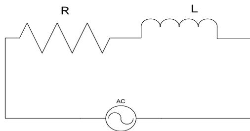
*Figure 1. A simple R-L circuit*
