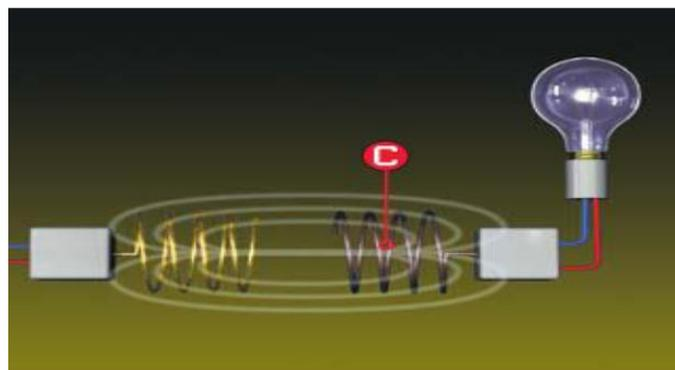
The energy of the oscillating magnetic field induces an electrical current in the receiving coil, lighting the bulb [D].
