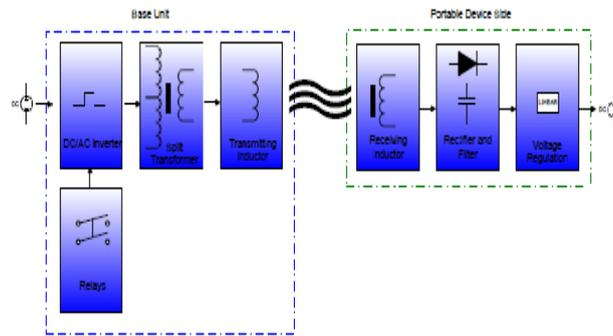
A circuit [A] attached to the wall socket converts the standard 60-hertz current to 10 megahertz and feeds it to the transmitting coil [B]. The oscillating current inside the transmitting coil causes the coil to emit a 10 -megahertz magnetic field
