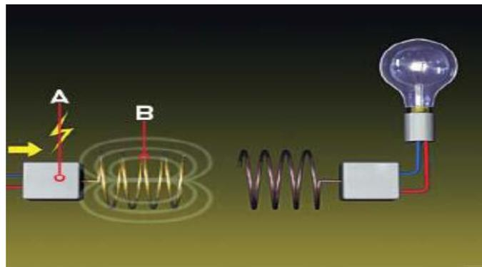
The receiving coil [C] has the exact same dimensions as the sending coil and thus resonates at the same frequency and, in a process called magnetic induction, picks up the energy of the first coil's magnetic field.
