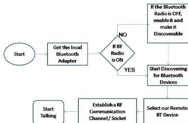
*Fig 4. Program Flowchart for establishing Bluetooth Connection*
