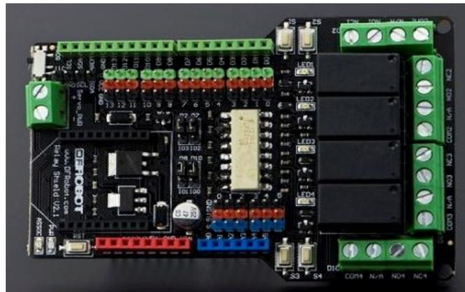
*Fig 3. Relay Board*
