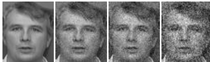
Fig.5 (a) face image before adding noise (b) Noisy image with SNR 15dB (c) Noisy image with SNR 12dB (d) noisy image with SNR 7dB
