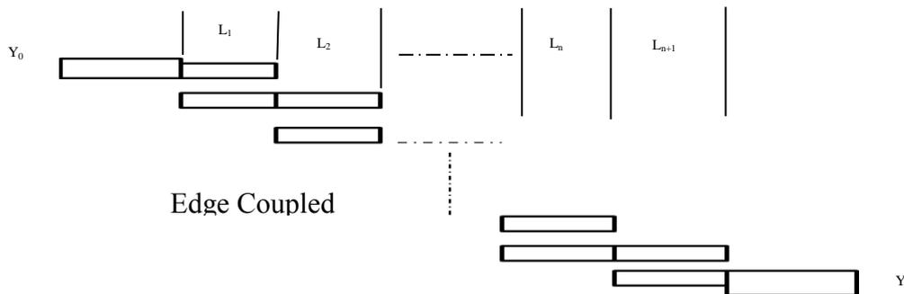
Fig. 3 General structure of parallel (edge)-coupled microstrip bandpass filter
