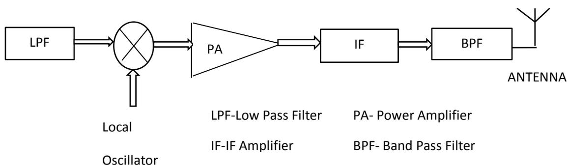
*Fig.1 Generic block diagram of Transmitter*
