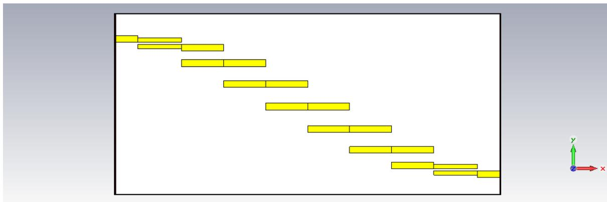
**Fig. 4 realized structure of Edge-Coupled microstrip bandpass filter**
