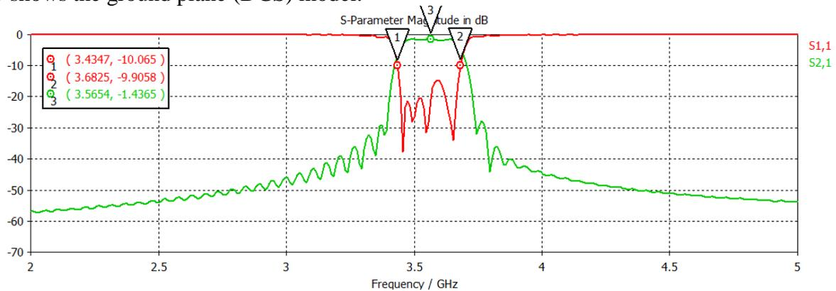
Fig. 6 Return Loss and Insertion Loss Results
