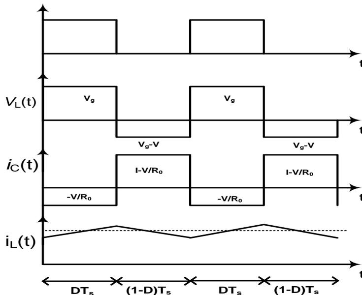
**Fig. 4. Waveforms of operation for Traditional Boost Converter connected to PV cell**
