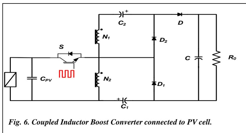
*Fig. 6. Coupled Inductor Boost Converter connected to PV cell.*
