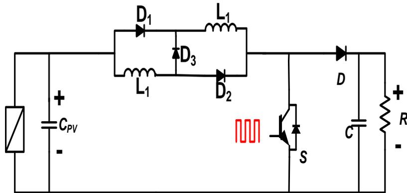
*Fig. 5. Switched Inductor Boost Converter connected to PV cell.*
