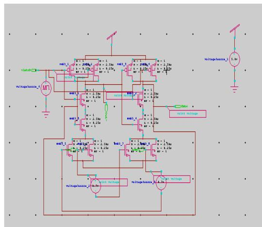
**Figure.5. Schematic design of Conventional Comparator**
