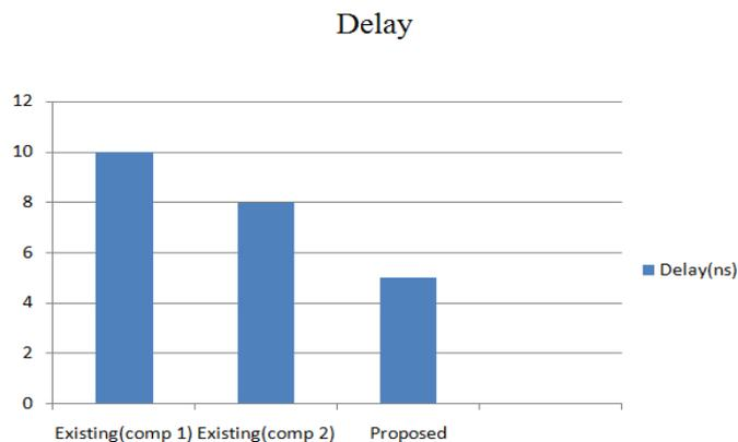
The above bar graph shows the relation between the delay obtained in various comparators. The frequency kept for all these transistors are 25MHZ.
