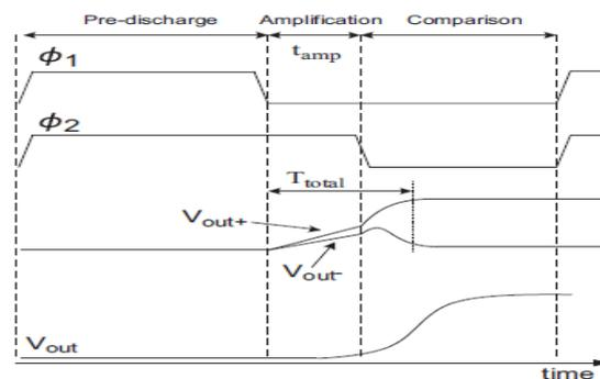
**Figure.3. Conceptual Waveform**
