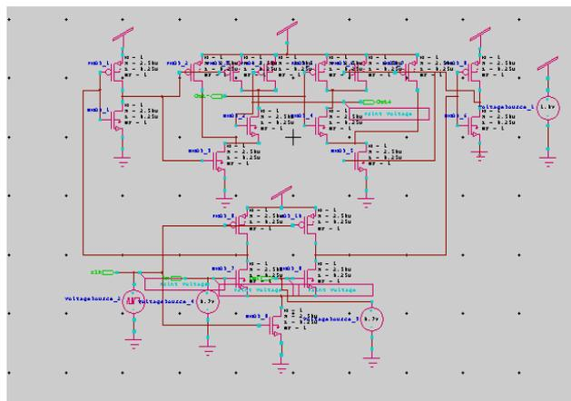
Figure.9. Schematic Design of Proposed Dynamic Comparator
