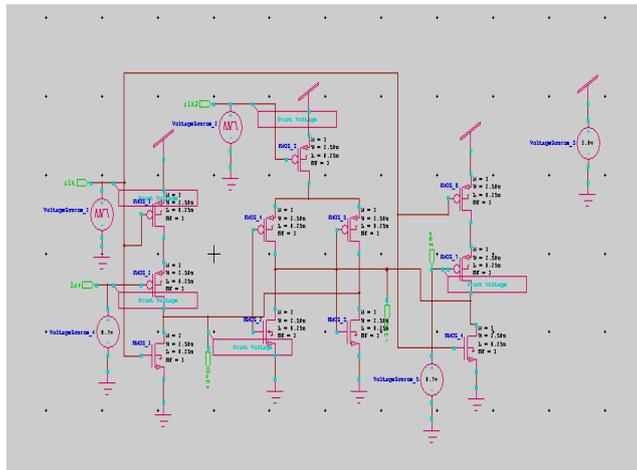
Figure.7. Schematic Design of Dynamic Comparator
