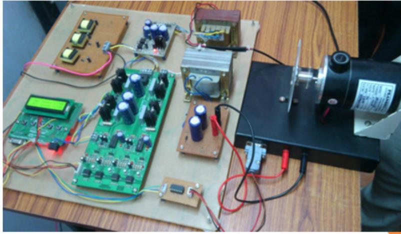
Fig. 7 Quasi Z Source network based DC Drive Hardware Setup
