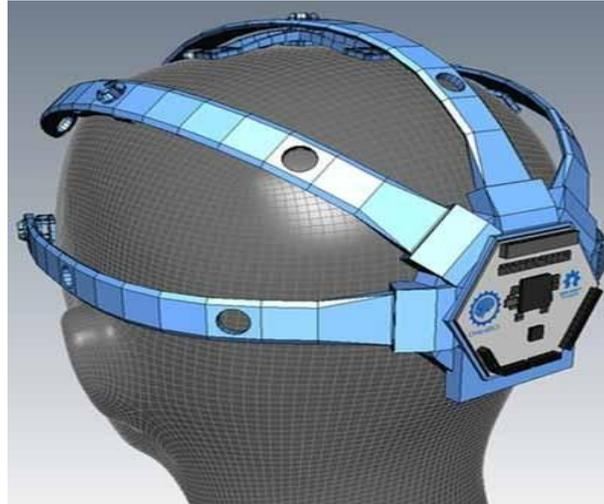
Fig4. OpenBCI wearable sensors and onboard computer
