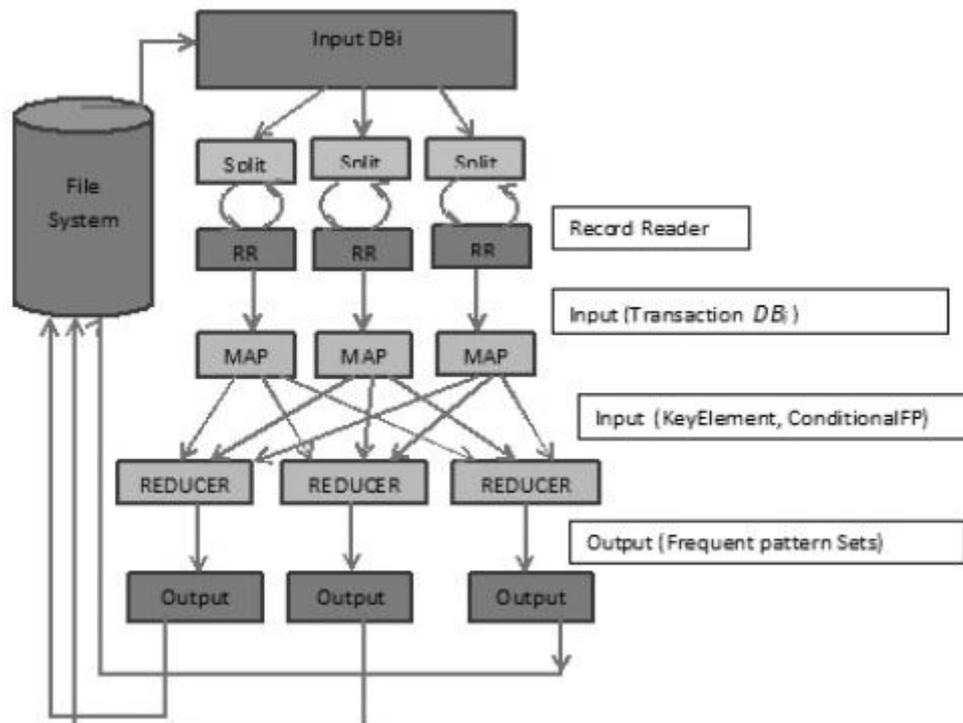
Figure 4. Architecture diagram of DPFPM algorithm using MapReduce framework
