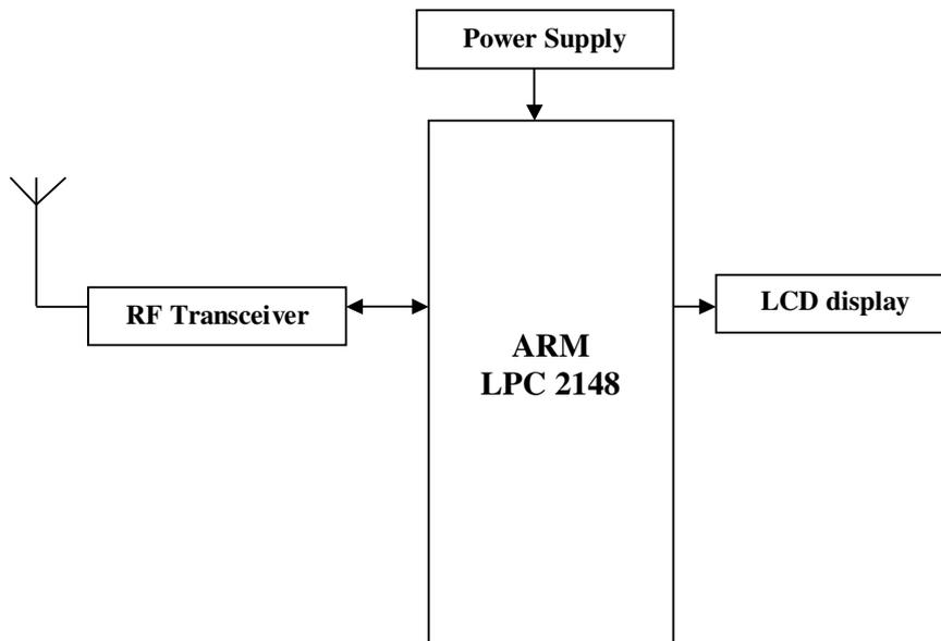
*Figure 4. Block diagram of monitoring section*
