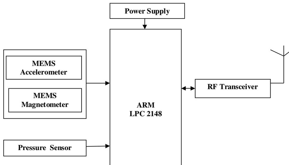
*Figure 3. Block diagram of Soldier's Section*
