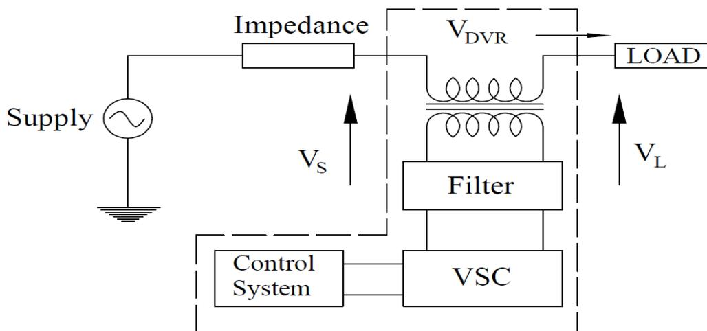
**Figure 3: Schematic diagram of DVR**
