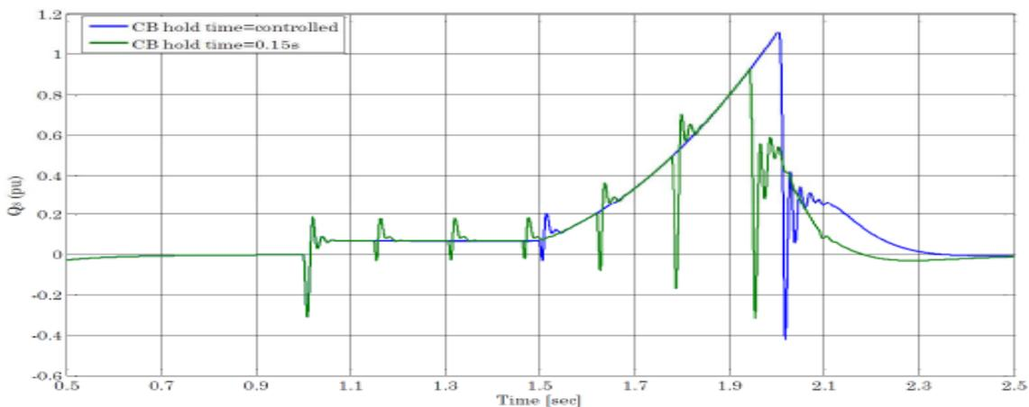
**Figure 11: Reactive power with different crowbar locking-times**
