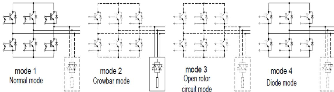
**Figure 6: Operation modes of DFIG Converter during FRT**
