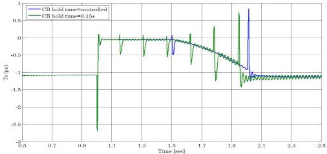
**Figure 12: Electromagnetic torque with different crowbar locking-times**
