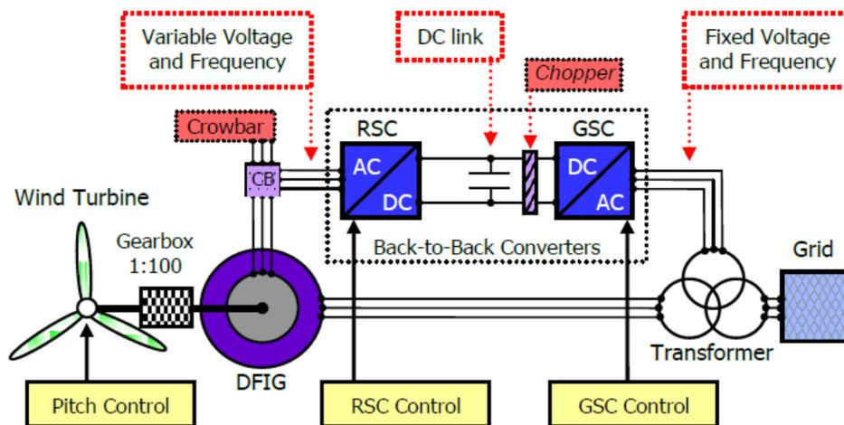
Figure 5: Basic operation of DFIG
