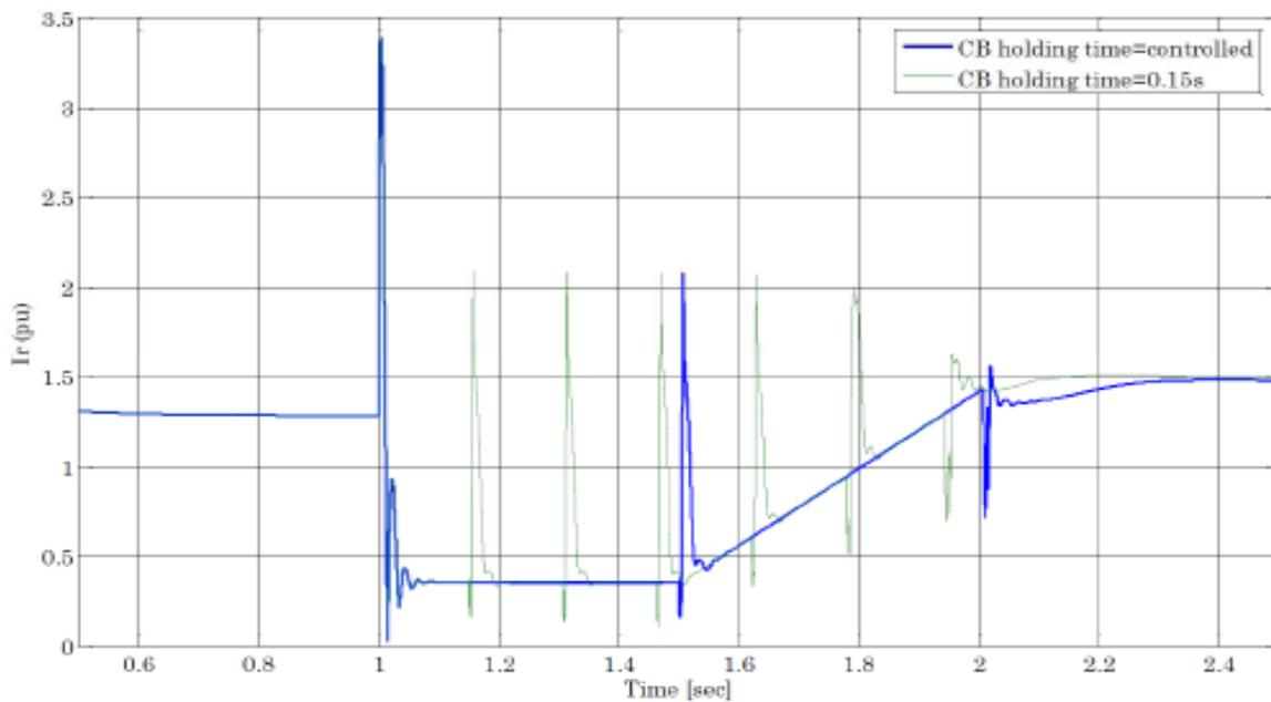
**Figure 10: Rotor current with different crowbar locking-times**
