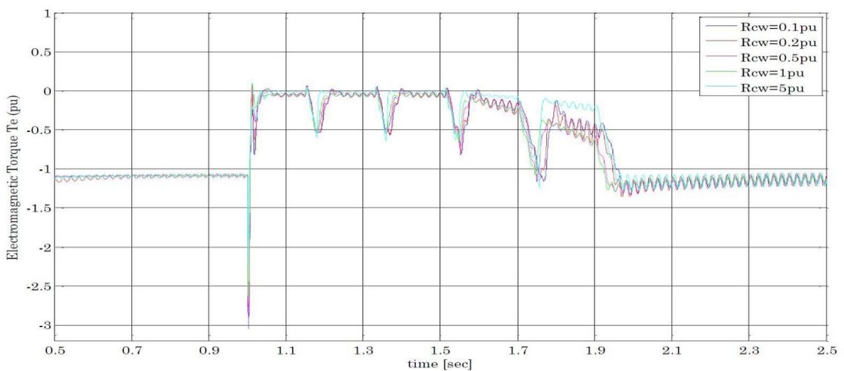
**Figure 9: Electromagnetic torque with different crowbars applied**
