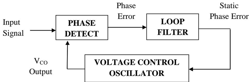
**Figure 2: Block diagram of an analog PLL**
