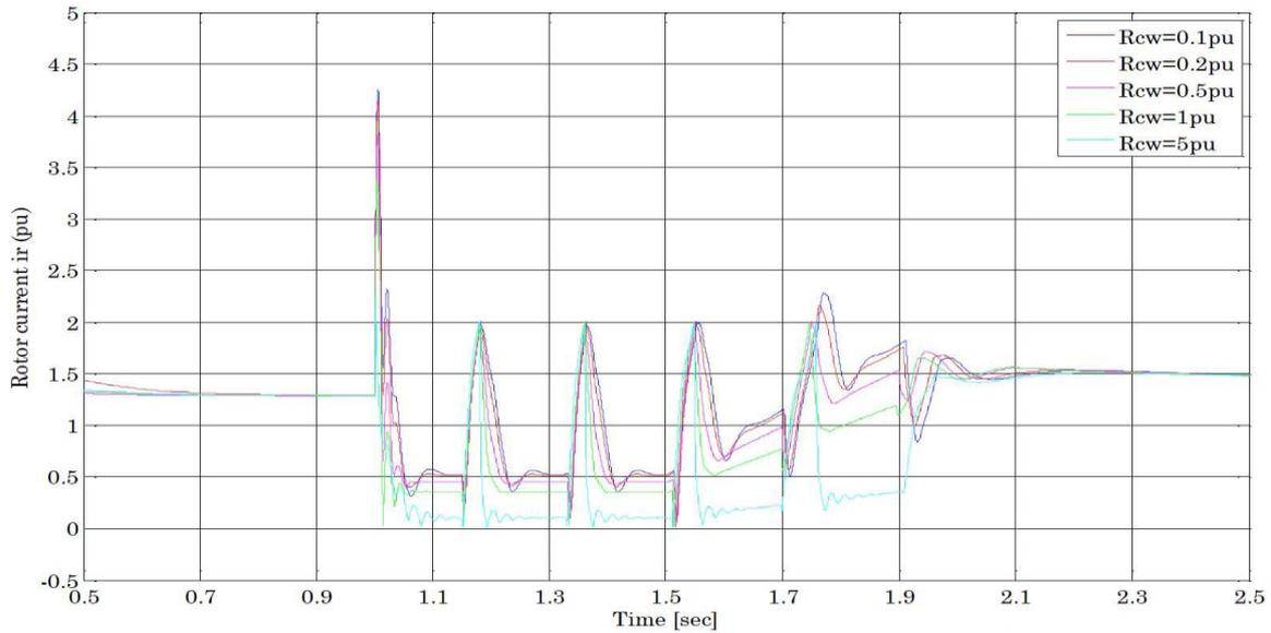
**Figure 8: Rotor currents with different crowbars applied**
